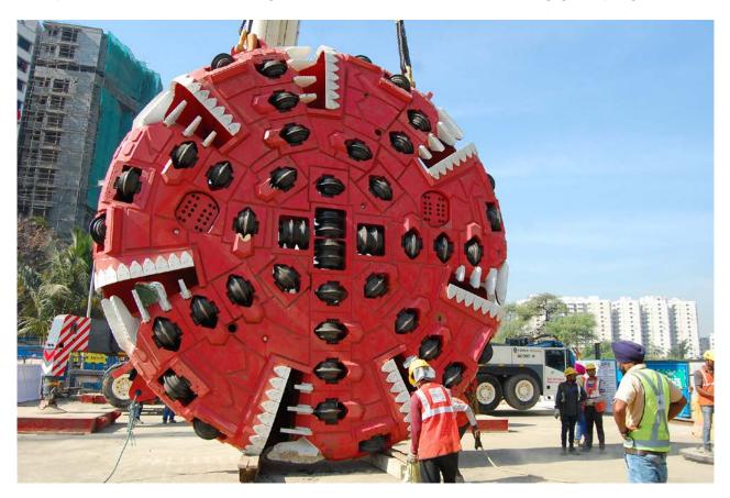
In early August, TERRATEC celebrated the assembly of its fifth new 6.68m diameter dual-mode hard rock Tunnel Boring Machine (TBM) to go to work on Mumbai Metro's Line 3 project, in India, at the CSIA International Airport shaft on contract UGC-06. The first four of these machines are now fully up and running on two other contract packages (UGC-02 and UGC-05) and achieving production rates of up to 91m per week, despite still being within the 'learning curve' period of their initial drives.
